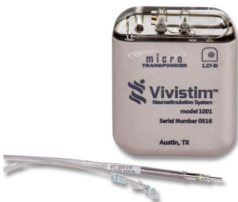
Figure 6.1: Vivistim ® System IPG and Lead
