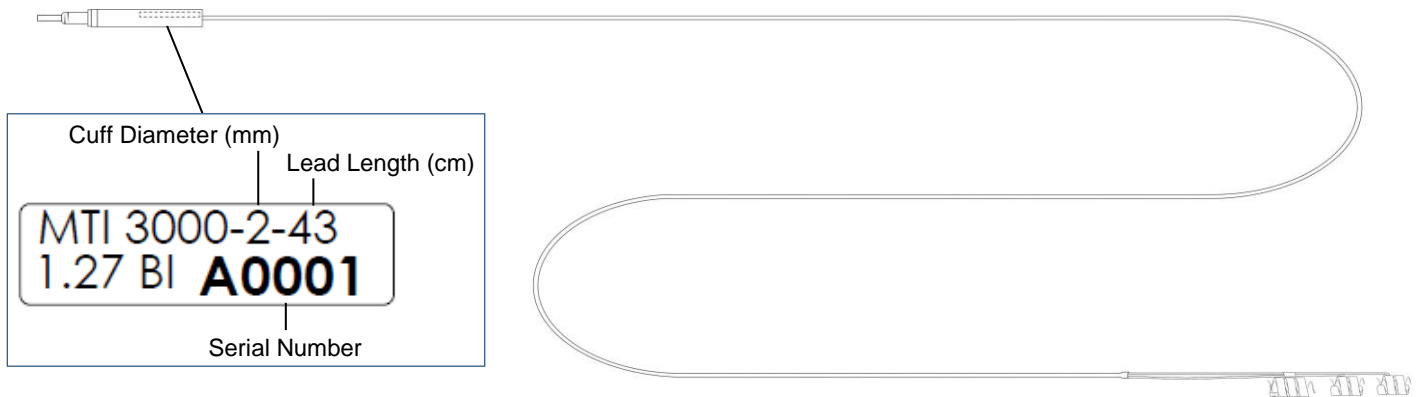
Figure 8.1: VNS Lead and Lead Identification Tag
